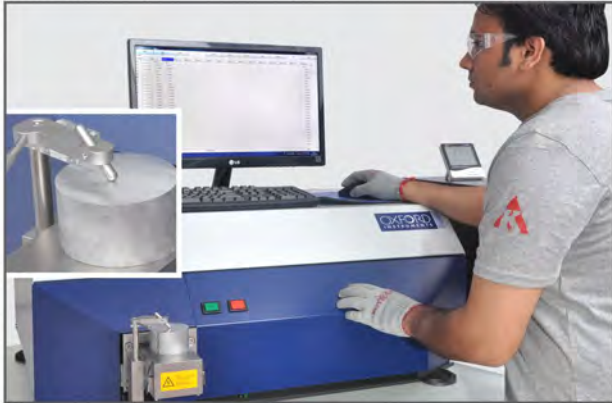
Testing of basic raw material rods/ sheets for correct composition on spectrometer.
